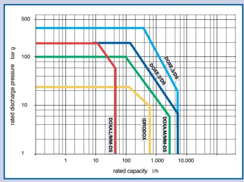
these diagrams give a general overview of available pumps and their performance range and can be used to select the model suitable for your application; for a more accurate selection and in case of particular process requirements, we recommend that you contact either OMG sales offices or your local OMG representative
